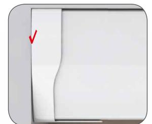
6. The endcaps can move outwards 10mm at each side, which can take up any small gaps between the headrail and the side of the recess that may appear due to mis-measurement.
