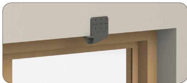
3. Centre supports are recommended on blinds over 600mm in width and should be fitted no more than 500mm apart. If centre supports are required, move the tool along the recess and drill required holes.
