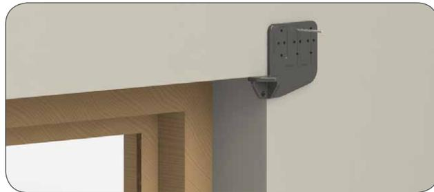
2. Pick the required overlap; 22mm (marked 'recess fit'), 50mm or 75mm. Keeping the tool in place, drill into the fitting surface using a 3mm bit through 2 of the 4 holes. *It is recommended to use the top and bottom holes where possible.*
