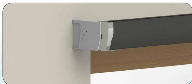
5. When all brackets have been fitted, insert blind by lining up fascia end caps with slots on fixing brackets. Adjustment of fascia end caps can be used to aid this process. When both sides have been located ensure blind is pushed fully home until locks on both the fixing and centre support have been snapped into place.
