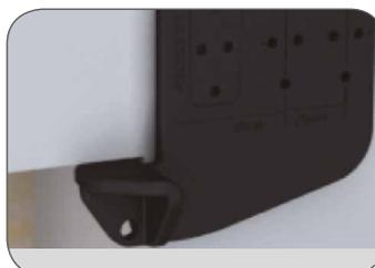
2. When face fitting, butt the square edges of the tool into the window recess, so that the arrows point horizontally away from the window as above.
